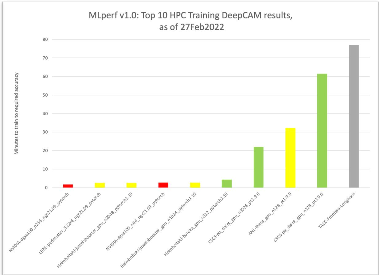
Figure 1 Top 10 MLperf v1.0 HPC DeepCAM training results
